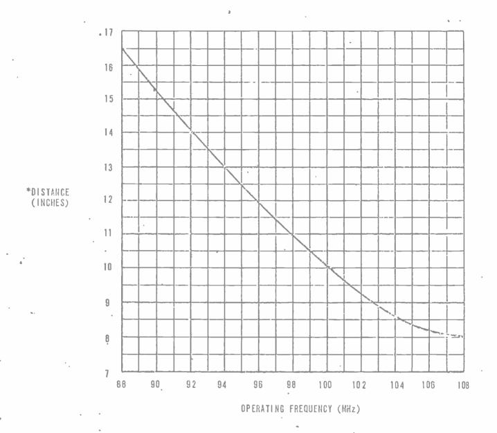
\*DISTANCE FROM THE PA TUBE DECK TO THE BOTTOM OF THE ROTARY SECTION OF THE PLATE CIRCUIT
