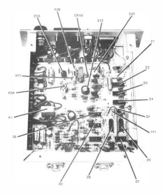
INTERNAL VIEW (OVEN COVER REMOVED) AFC UNIT FIG. 4.4
